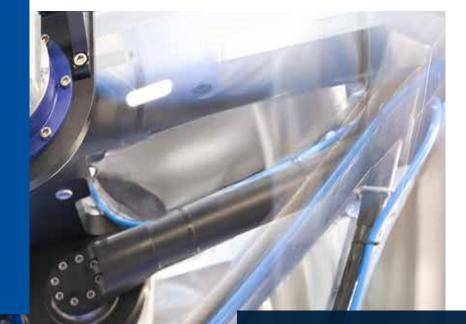
As the most flexible component of a machine, the Delta robot is the first choice for customized production. This supports fast sorting according to cell quality levels and precise alignment on the moving conveyor belt at the end-of-line quality gate.
