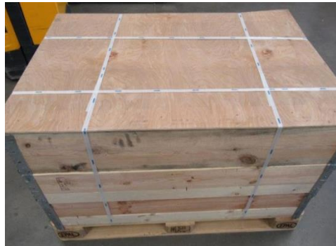
Figure 5 EPAL Euro pallet with 3 pallet frames, a wooden cover and 4-fold banding.
