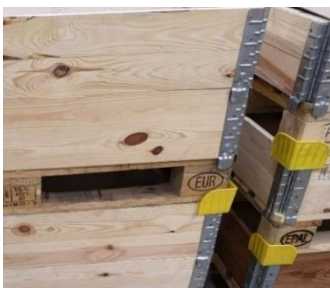
Figure 6 Securing the stack of pallets with hinged frames using stacking corners
